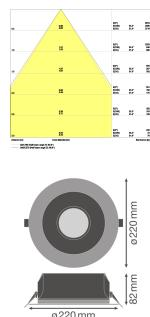
**Scheda tecnica Ledvance Downlight LED Performance DN195 21W 2400lm 65D - 830 Luce Calda | 220mm - IP54 - Dali Dimmerabile**
