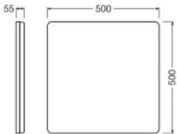
**Scheda tecnica Ledvance Bulkhead LED Surface Piatto Fonti luminose Piazza Bianca 23W 3780lm - 830-840 CCT | 500mm - IP20**
